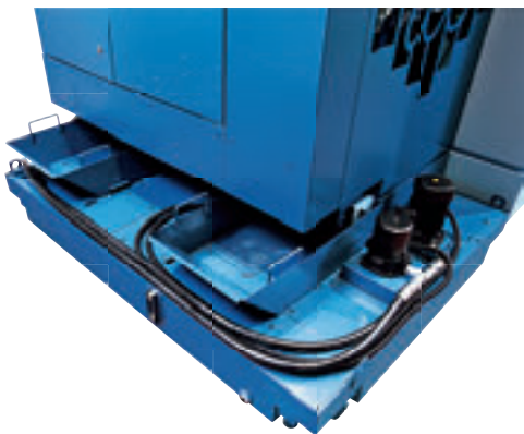
Standard Coolant tank
