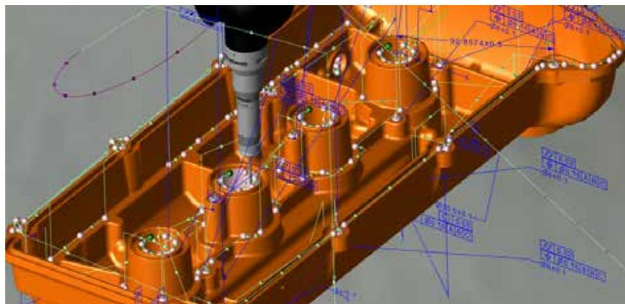
MiCAT Planner prevents risk of misinterpretation: each GD&T symbol, tolerance and datum is automatically understood and converted in the corresponding required measurement points. In the program view, all GD&T are shown in regards to the feature to be measured for calculating the result.
