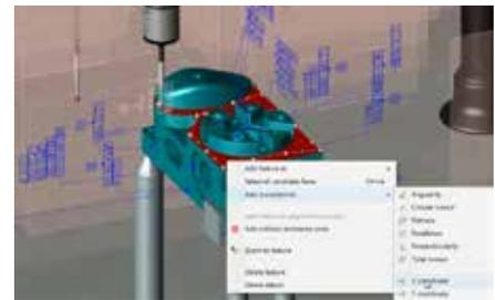
If required, a missing feature (not identified on the CAD model) or a missing characteristic to be evaluated can be manually added from the 3D view.
