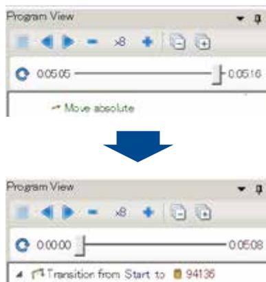
MiCAT Planner automatically estimates the measuring cycle time according to the actual CMM configuration and settings. For example, the required time for exchanging a probe in the rack, or the specified scanning speed in your measurement rules, are considered for this time estimation. Immediately after the cycle optimization is executed, the new estimated cycle time is displayed.
